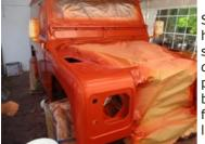
So now we are in April, Phoenix wasn't in great shape as he needed a lot of panel fettling with aluminium fillers and special zinc primer to hold the corrosion. Once the major dents were pulled out and re-riveted, the 3 coats of filler primer was applied wet and drying between all coats, the base of the orange mid part of the orange and then the final drop coat of the orange was applied and then 3 lacquers... yes 3!
